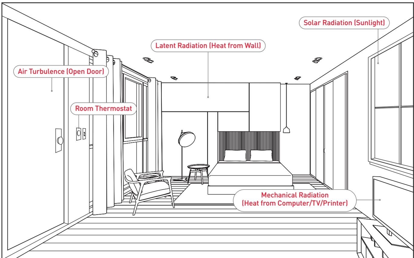
While thermostat placement may appear straightforward, no matter how hard the designer tries, it often ends up in the wrong location; wrong in the sense that it doesn't achieve its primary function. The thermostat fails because it's measuring the temperature of the wall and not the occupants in the room. With a wall-mounted thermostat, the wall may be comfortable, but not the occupants.
