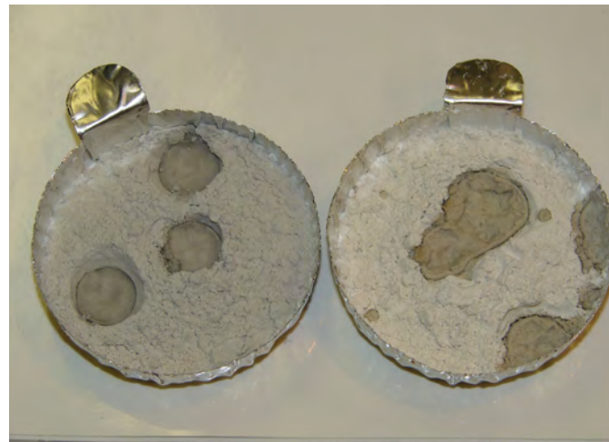
Wetted silica dust takes on the characteristics of mud, as shown in these samples. A dry environment should be maintained whenever possible to prevent the muddy dust from clogging filters.
